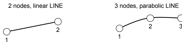
Figure 2a Schematic representation of the 1-D finite element types implemented in HEATER.
